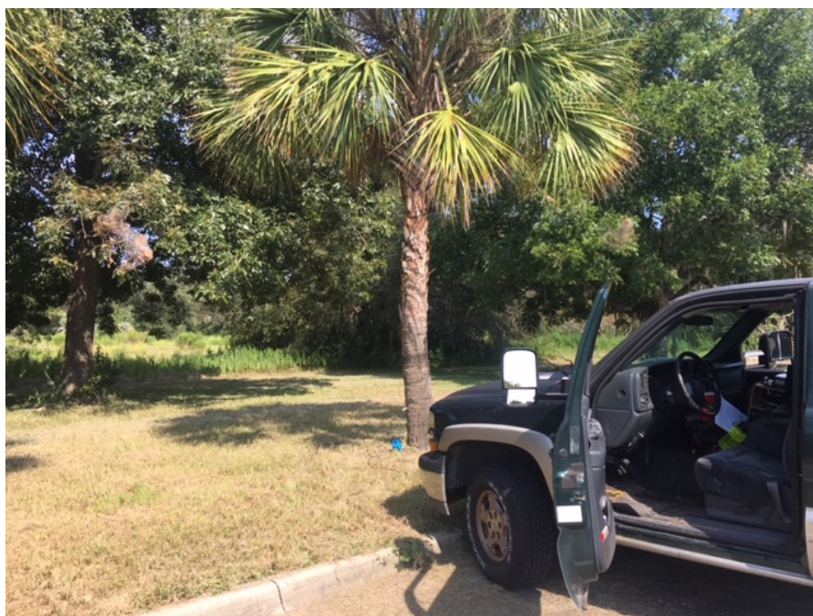
Monitoring Station Location. Wire vertical came down in the palm tree. Blue box visible at the bottom of the palm is the 1:49 end-fed balun in a Carlon electrical handy box.
